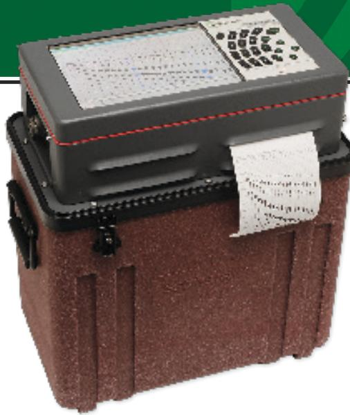
For those practitioners who prefer not to use laptops in the field, the feature-packed StrataVisor NZXP is an “all-in-one” seismograph housed in a compact, weatherproof and shockproof chassis. In addition to a built-in PC, it includes a brilliant daylight-visible color screen, waterproof keypad and built-in printer.
