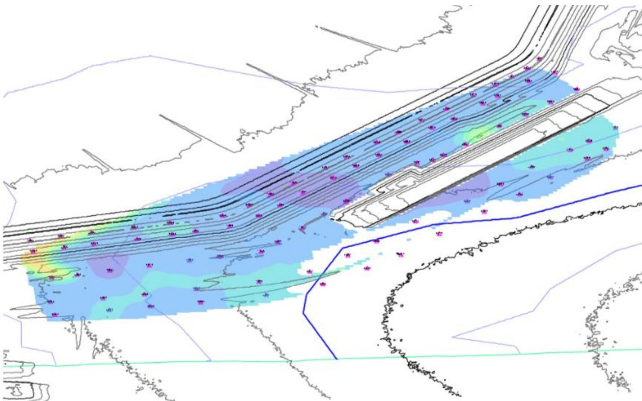
*Dense surface arrays can be used to image the subsurface within TSFs. A horizontal slice through the 3D model is shown in colour scale at the level of the toe. Low velocity zones (blue) indicate seepage pathways through the structure to the seepage pond.*
