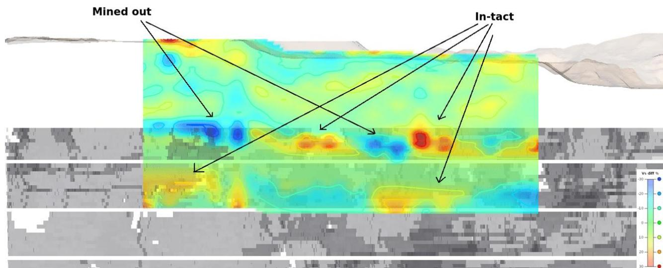
Other applications of ANT in a geotechnical context typically involve the detection of voids or cavities. Where in-mine seismic systems exist, the resolution of the model can be enhanced using travel-time tomography.
